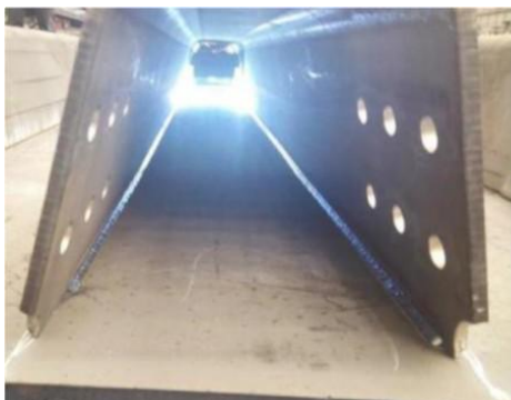
a) Fully mechanized weld inside the stiffener Figure 4. Double-sided weld
