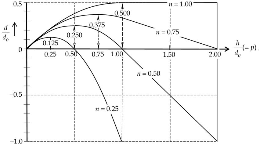
Figure 8. Relation between water level  $d$  and the water column  $h$  for low  $n$ -values of sloping roofs
