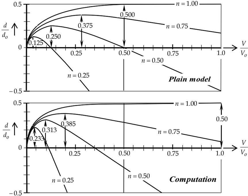
Corresponding graphs in the two figure parts have roughly a similar shape. The correspondence is close for  $n$ -values near 1.00, and less for  $n \leq 0.50$ . The water raising capacity of each graph is shown in the picture. Comparison of the two figure parts justifies the conclusion that the raising capacity of the computational analysis is always larger than predicted by the plain model. This supports the statement that the model is conservative.
