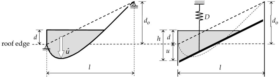
Figure 6. Modelling of the real sloping beam (left-hand picture) to the inclined piston-spring model (right-hand picture)
