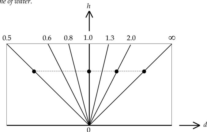
Figure 4. Relation between water column  $h$  and water level  $d$  for different  $n$ -values
