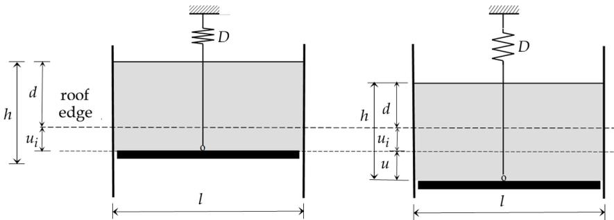
Figure 14. Extension of model for slope-less flat roof by initial displacement  $u_i$  due to permanent load. Left: Undeformed. Right: Deformed. Left and Right: Same water column  $h$ .
