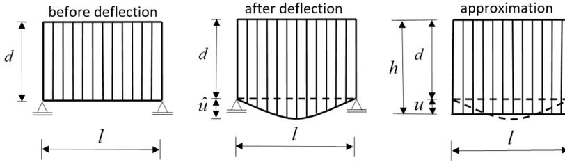
Figure A1. Undeformed beam (left). Deformed (mid). Idealized waterloading (right)
