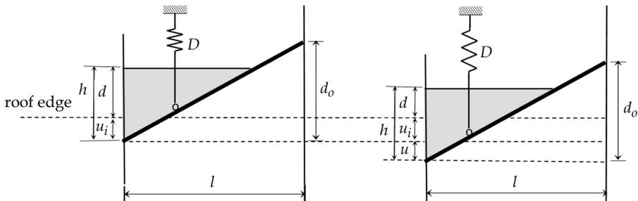
Figure 15. Extension of model for sloping flat roofs by initial displacement  $u_i$  due to permanent load
