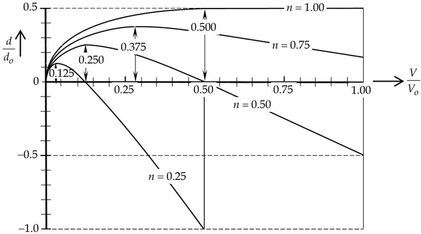
Figure 11. Relation between  $d$  and the volume  $V$  of sloping roofs for different values  $n \leq 1$
