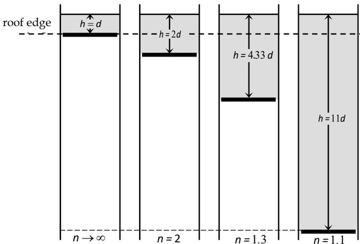
Figure 3. Water column  $h$  for decreasing stiffness ratios  $n$  (same discharge position)
