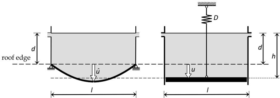
Figure 1. Modelling of the real beam (left-hand picture) to the piston-spring model (right-hand picture)
