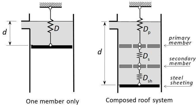
Figure 16. Composed model of primary members, secondary members and profiled steel sheeting
