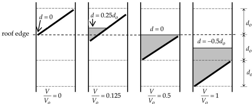
Figure 12. Position of piston and measure of water filling for four volumes, for  $n = 0.5$
