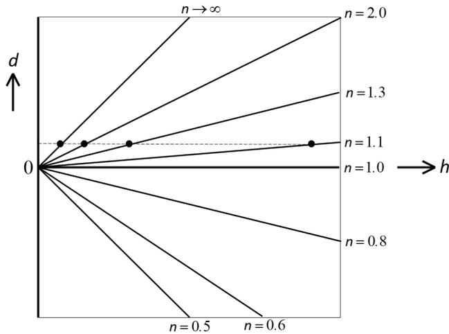
Figure 2. Relation between water level  $d$  and water column  $h$  for different  $n$ -values of flat roofs
