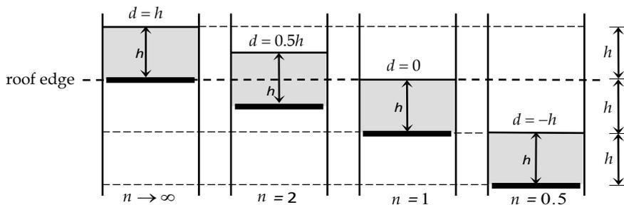
Figure 5. Water surface  $d$  for decreasing stiffness ratios  $n$  (same water column  $h$ )
