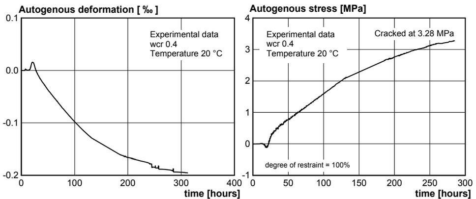
Figure 11: TSTM results for a free deforming specimen and a fully restraint specimen due to self-desiccating stresses, also indicated as autogenous stresses, under sealed conditions [4]
