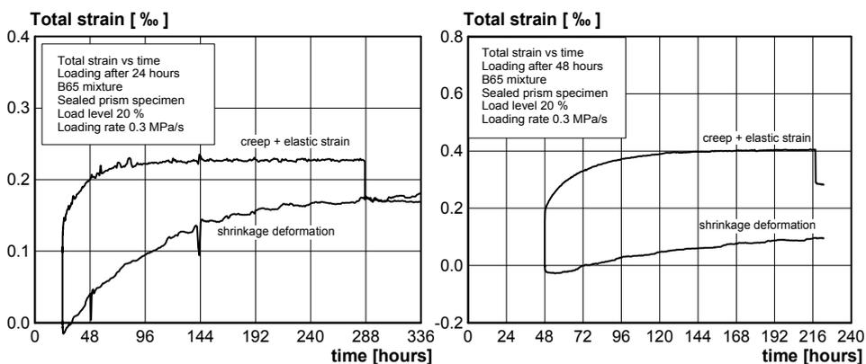
Figure 18: Total strain results (elastic + creep) measured on a sealed prism specimen loaded (20%) after 24 and 48 hrs of age, and load independent shrinkage strain measured from control specimen
