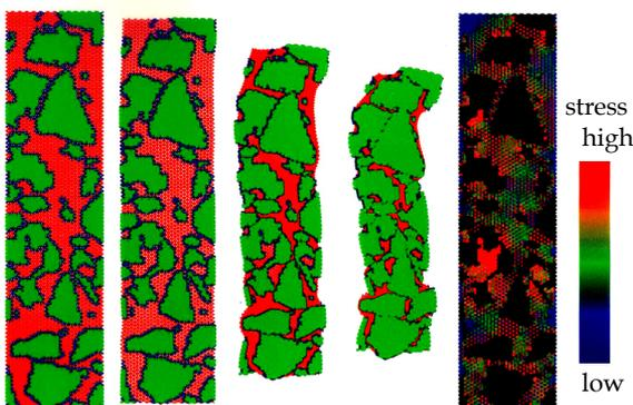
Figure 9: Schematic representation of autogenous deformation of a prismatic concrete specimen. Left: Four sequential steps showing the progressive development of autogenous deformation, and Right: The corresponding tensile stresses that developed in the cement paste [4]
