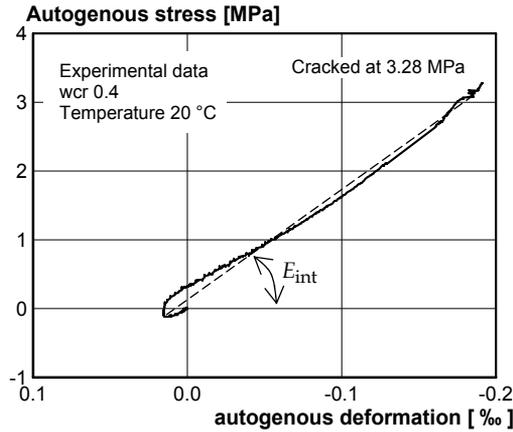
Figure 12: Autogenous stress versus autogenous strain measured on a full restraint TSTM specimen, under sealed conditions and constant temperature of 20 °C [4]
