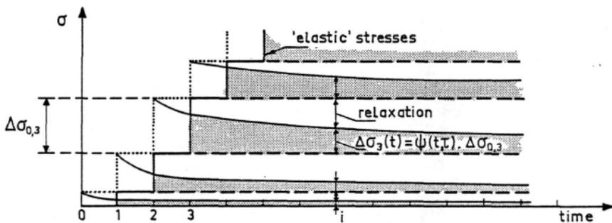
Figure 3: Schematic representation of the evolution of a temperature curve, an elastic modulus and the superposition of incremental stresses [1]
