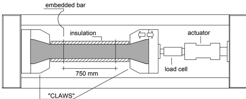
Figure 10: Schematic representation of a Thermal Stress Testing Machine (TSTM) for measuring self-desiccating stresses or deformations on sealed and thermally controlled hardening specimens
