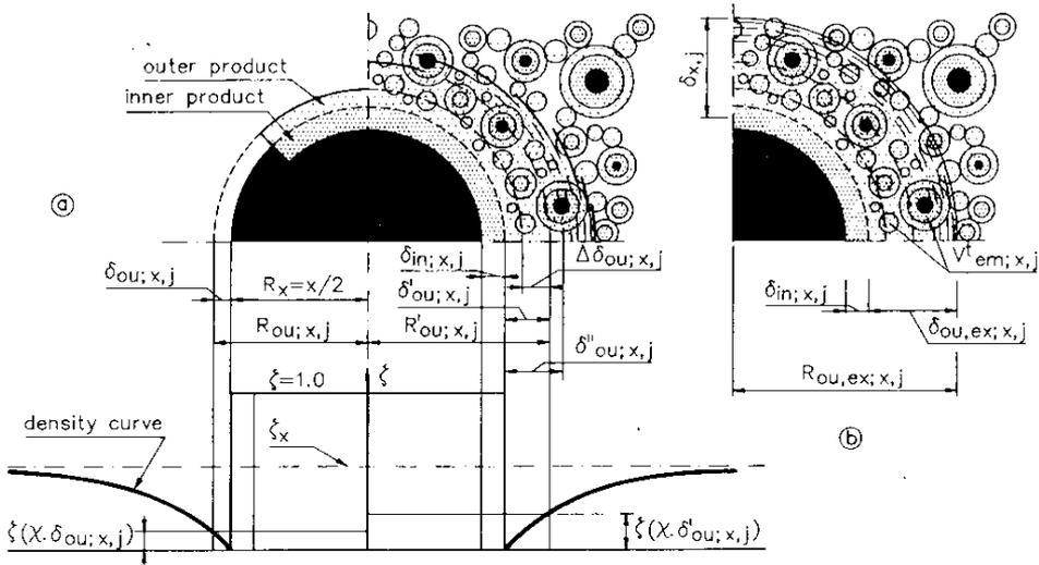
Figure 5: Particle expansion mechanism of the HYMOSTRUC model proposed by Van Breugel [2]
