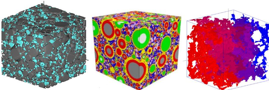
Figure 6: Results of HYMOSTRUC model. Left: Blended particle structure at initial stage [10]. Middle: Blended particle structure after hydration has ceased [9]. Right: Transport of capillary water through the developing pore structure of the hydrating microstructure [11]
