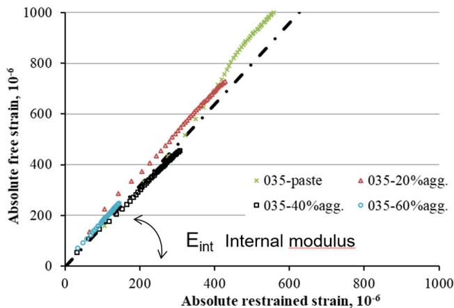
Figure 13: Autogenous stress versus autogenous strain for various concrete mixtures showing a constant linear elastic constitutive behaviour [13]
