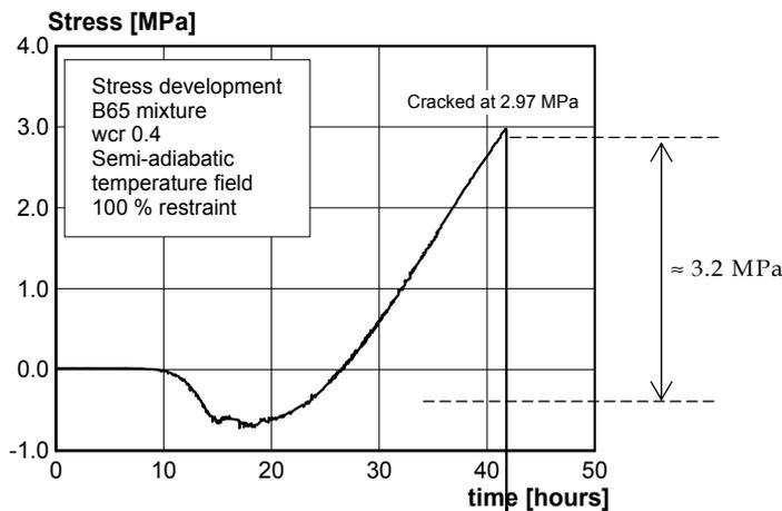
Figure 15: Stress development with time in the considered TSTM specimen under sealed conditions
