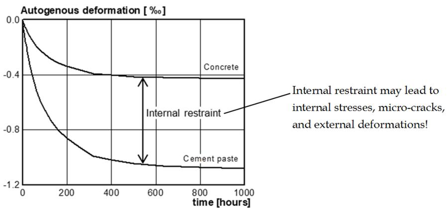
Figure 8: Schematic representation of autogenous deformation of cement paste without aggregates and of concrete with aggregates added. The difference in deformation shows internal restraint [4].
