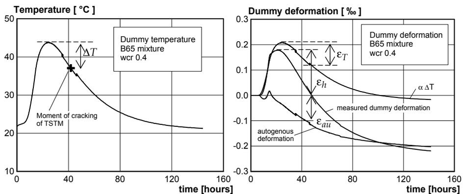
Figure 14: Left: Semi-adiabatic temperature development measured in the TSTM specimen during hardening. Right: Autogenous shrinkage strains and total load independent deformation that developed during hardening in the complementary dummy (control) specimen [15]
