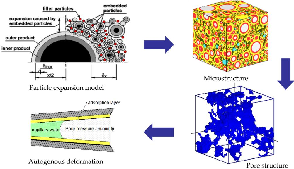
Figure 7: Schematic representation of the built up from particle structure, to microstructure, to pore structure, to internal capillary stresses and autogenous deformation
