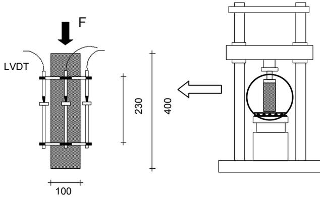
Figure 16: Creep setup with a detailed view of the LVDT configuration. For both the control and the creep specimen, the deformations were measured with a similar LVDT configuration [15]
