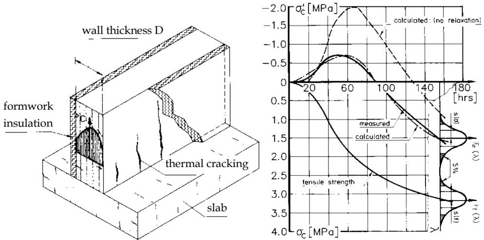
Figure 4: Left: Schematic representation of a wall with early age cracks. Right: Stress and strength development in an early age hardening concrete element [2]
