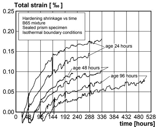
Figure 17: Load independent deformations of prism specimens. Measurements started after 24, 48 and 96 hours of age, sealed conditions [15]
