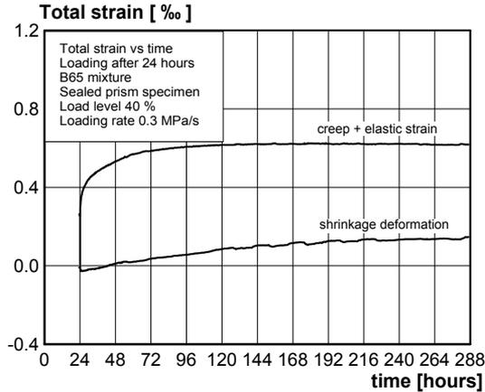
Figure 19: Total strain results (elastic + creep) measured on a sealed prism specimen loaded (40%) after 24 hrs of age, and the load independent shrinkage deformation from the control specimen
