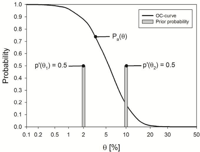
Figure 2: OC-curve and prior probabilities for the basic example
