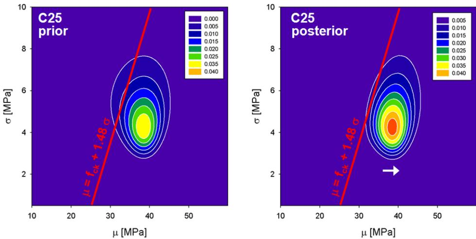
Figure 4: Contour plot of the prior (left) and posterior (right) joint density function of the parameters for the concrete strength distribution corresponding to a concrete class C25 after conformity control based on the conformity criteria under consideration
