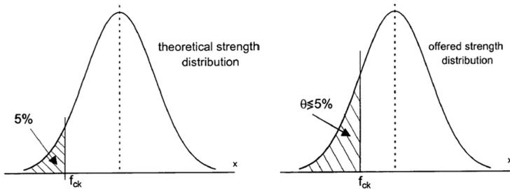
Figure 1: Theoretical and offered strength distributions in case of concrete compressive strength
