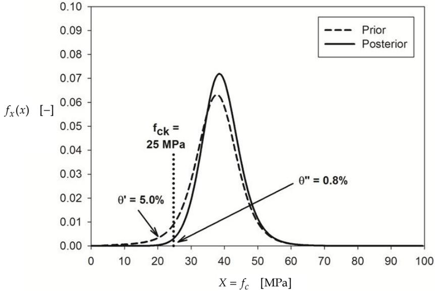
Figure 5: Prior and posterior predictive concrete strength distributions for a C25 concrete class after conformity control based on the conformity criteria under consideration
