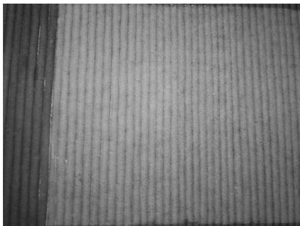
*Figure 5: Test panel A considered to be the right 'end product' by the cleaning company themselves. The slightly lighter coloured part in the middle was pre-cleaned by dry microblasting prior to laser, the right part was cleaned by laser only. At the leftmost part of the picture the non-cleaned black weathered sandstone.*
