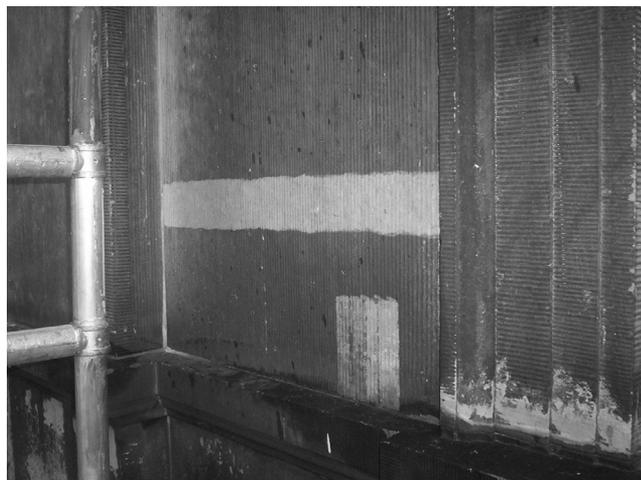
*Figure 7: Test panel C cleaned by laser*
