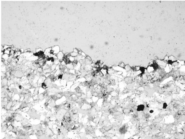
*Figure 16: Microphotograph showing the partial cleaning obtained by laser on test panel C, with some material of the black weathering layer remaining in deeper pores and behind quartz grains (sample TNO 00426, plane polarized light, view 2.7 x 1.8 mm)*
