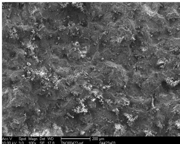
*Figure 11: SEM microphotograph of the surface of non-cleaned Obernkirchen sandstone from test panel A (sample TNO 00422)*
