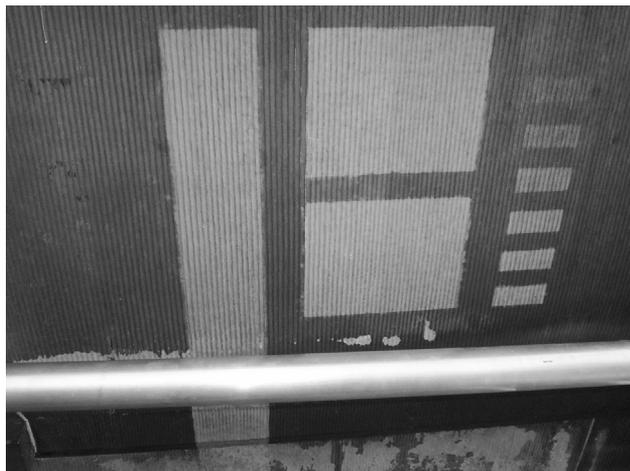
*Figure 4: Overview of test panels A. On the right, scale bar made to determine operating conditions of the laser. In the middle, test panels considered to be the right 'end product' by the cleaning company themselves. A detail of these is given in figure 5. For explanation, see text.*
