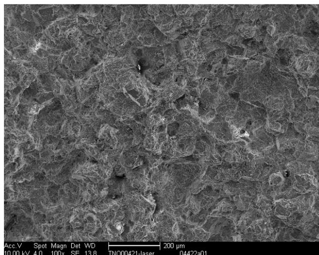
*Figure 13: SEM microphotograph of the surface of Obernkirche sandstone from test panel A cleaned by laser (sample TNO 00421)*
