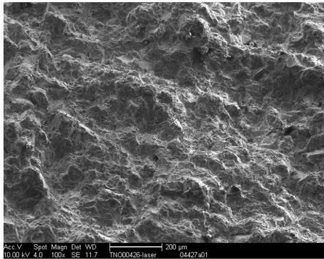
Figure 17: SEM microphotograph of the surface of Obernkirchen sandstone from test panel C cleaned by laser (sample TNO 00427)
