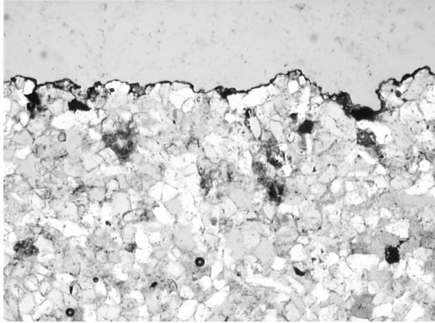
*Figure 15: Microphotograph showing the more continuous thin black weathering layer on non-cleaned Obernkirchen sandstone from test panel C (sample TNO 00427, plane polarized light, view 2.7 x 1.8 mm)*
