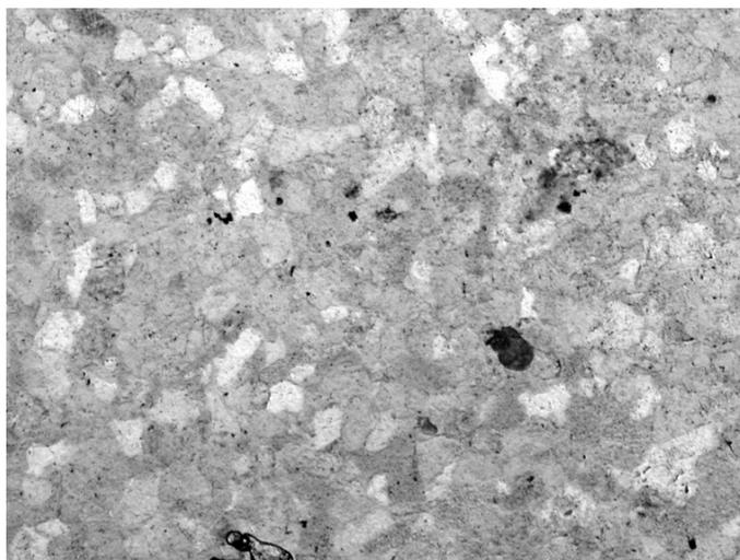
Figure 1: Microphotograph showing the microstructure of Obernkirchen sandstone (sample TNO 00245, plane polarized light, view 2.7 x 1.8 mm)
