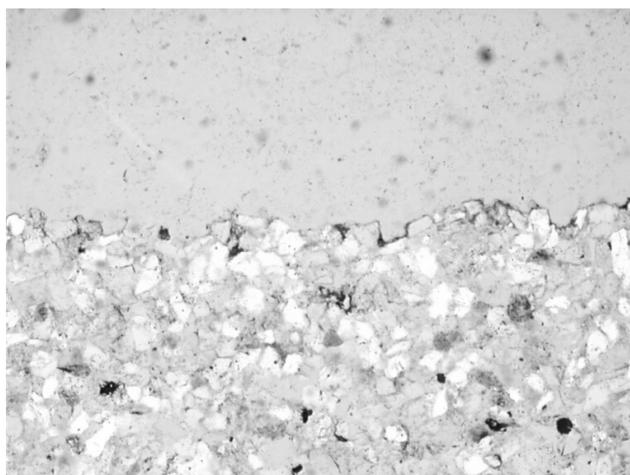
*Figure 10: Microphotograph illustrating the removal of the thin black weathering layer from the surface of the quartz grains after cleaning by laser, with some material remaining in the deeper pores (sample TNO 00421, plane polarized light, view 2.7 x 1.8 mm)*
