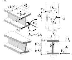
Figure 3: Displacements due to bending of the flange and warping of the profile
