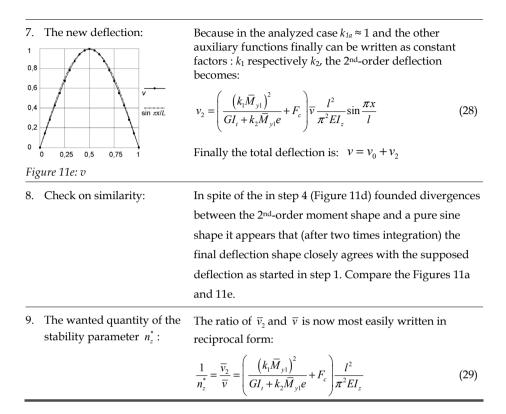
From (14) it follows that the amplification factor runs to infinity for  $n_z^* = 1$ . The situation then has become critical. We will consider three cases for which  $n_z^* = 1$  applies:
