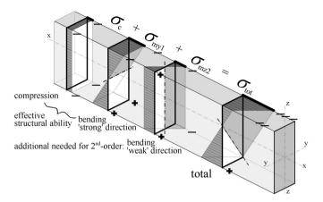
Figure 13: Superposition of stresses
