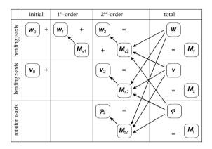
Figure 5: Interactions of displacements and moments
