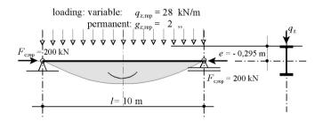
Figure 14 I-beam under representative uniform loading
