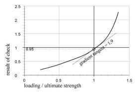
Figure 15: Increasing check result for increasing loading
