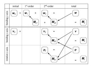
Figure 8: Reduced interaction scheme of displacements and moments
