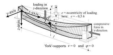
Figure 1: Structural member on two supports
