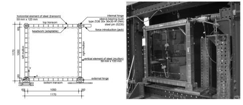
Figure 6: Test set-up (without beadwork)
