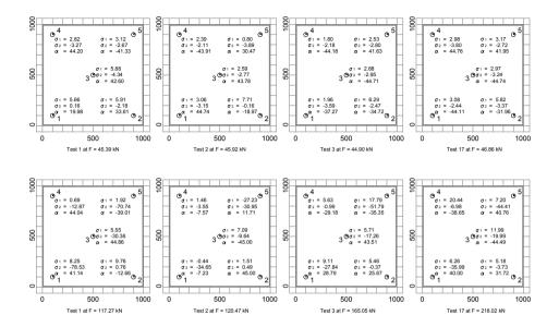
$\sigma_1$  is the maximum principle stress calculated from measured strains
