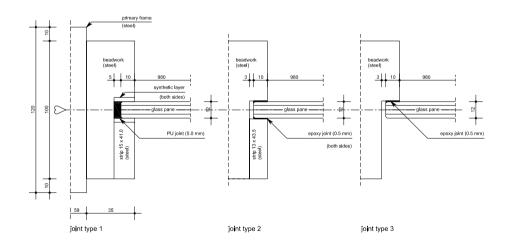
Figure 8: Beadworks belonging to joint type 1 to 3
