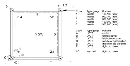
Figure 9: Position of measuring devices
