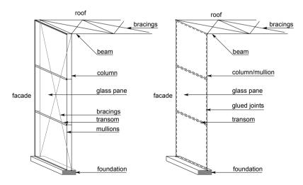
Figure 1: Separated main bearing structure and façade envelope (left) Integrated façade structure with glass panes as shear wall (right)
