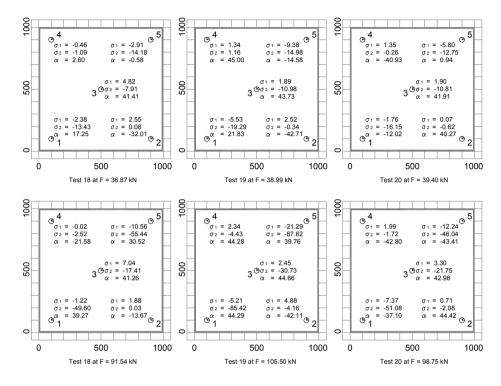
$\sigma_1$  is the maximum principle stress calculated from measured strains
