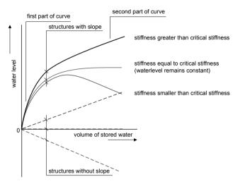
Figure 12: The relation between the water level and the volume of stored water for different stiffness
