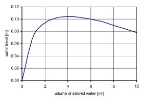
Figure 10: The relation between the water level and the volume of stored water
