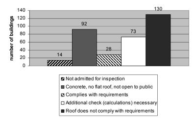
Figure 5: Inspection results for objects with flat roofs (Inspections carried out in the period 2004 – 2006)
