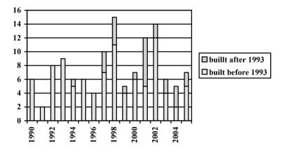
*Figure 1: Number of light-weight flat roofs yearly collapsed in the Netherlands due to rainwater ponding. 50% of the total estimated. (Source: Hageman [1])*
