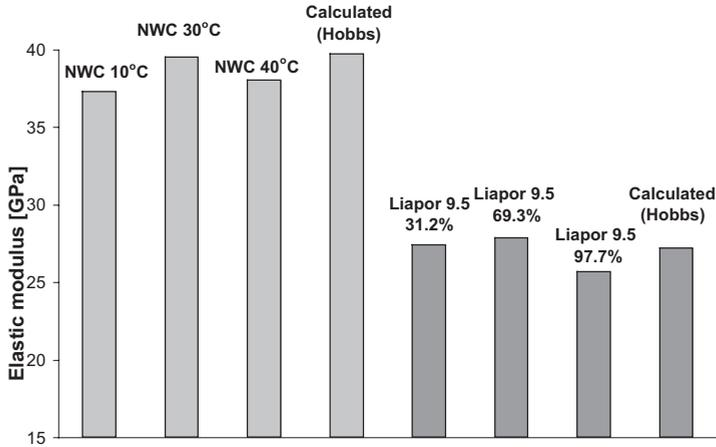
Figure 11. Measured and calculated 28-days elastic modulus of NWC (left, Mix C in reference [7], curing temperature 10, 30 and 40°C) and LWAC (right, mixes in Table 2, curing temperature 20°C)
