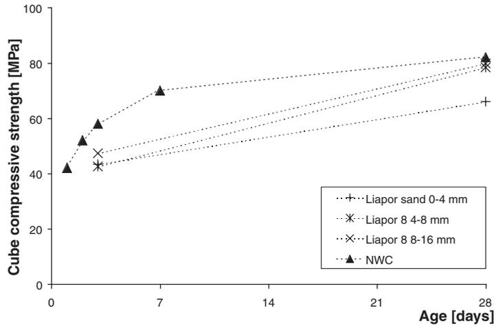
Figure 5. Cube compressive strength of LWAC with different particle size of the LWA compared with the corresponding NWC
