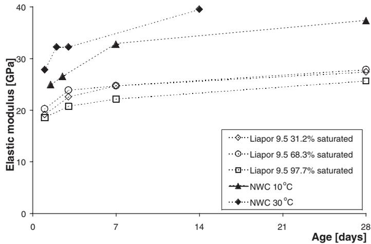
Figure 6. Elastic modulus of LWAC with different degrees of saturation of the LWA compared with the corresponding NWC
