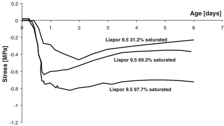
Figure 8. Self-induced stress of LWAC with different degrees of saturation of the LWA
