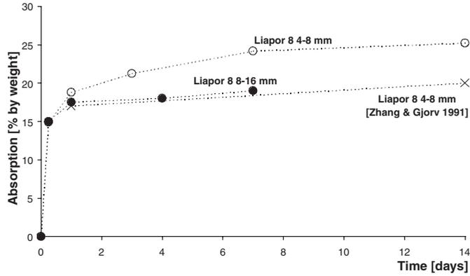
Figure 1: Percent water absorption by weight of Liapor 8, 4-8 mm and 8-16 mm fractions, stored in water at 20 °C
