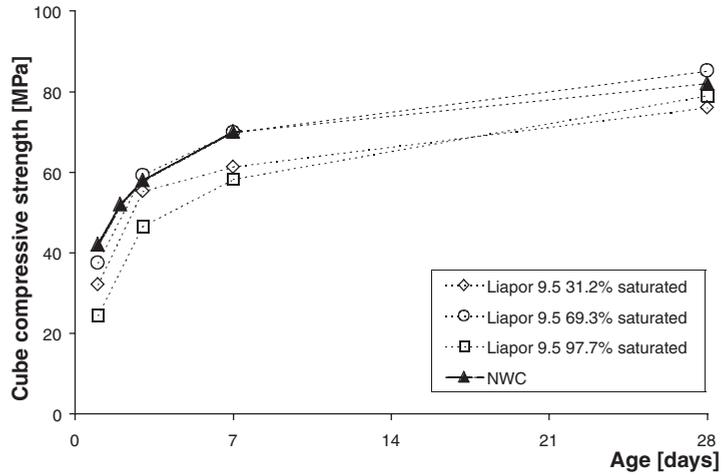
Figure 4. Cube compressive strength of LWAC with different degrees of saturation of the LWA compared with the corresponding NWC
