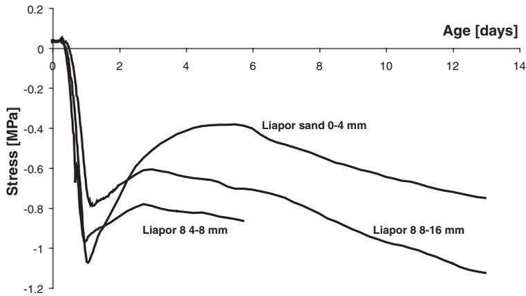
Figure 10. Self-induced stress of LWAC with different particle size of the LWA
