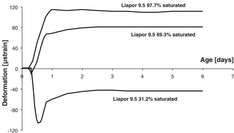
Figure 7. Autogenous deformation of LWAC with different degrees of saturation of the LWA
