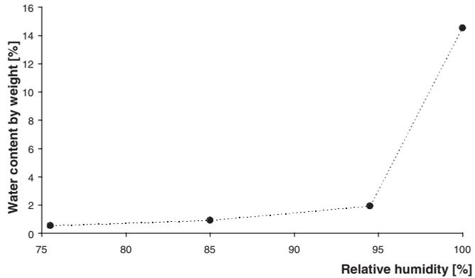
Figure 2. Desorption of Liapor 8 4-8 mm at  $20 \pm 1$  °C
