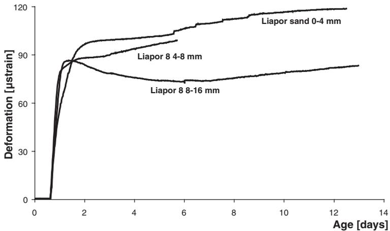
Figure 9. Autogenous deformation of LWAC with different particle size of the LWA
