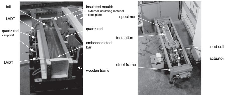
Figure 3. Left, experimental setup for the measurement of the free deformations of hardening concrete (ADTM). Right, experimental setup for the determination of stress development in hardening concrete (TSTM).
