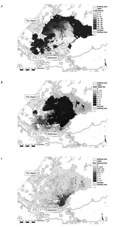
*Figure 2: Case study: flood characteristics computed with the 2D hydraulic model: (a) time of inundation (hours after failure of the river dike), (b) maximum water depth (m), (c) maximum flow velocity (m/s)*
