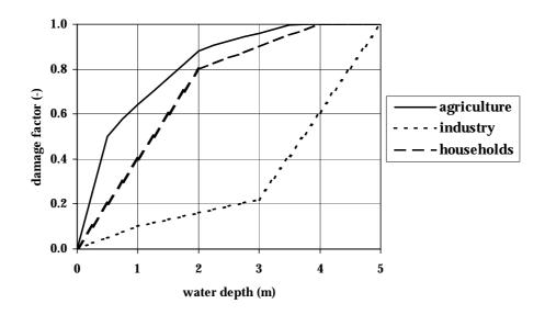
Figure 4: Example of damage function according to Standaardmethode (Kok et al. 2002)
