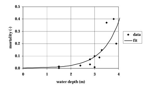
Figure 6: Proposed function for estimation of flood mortality for rapidly rising water
