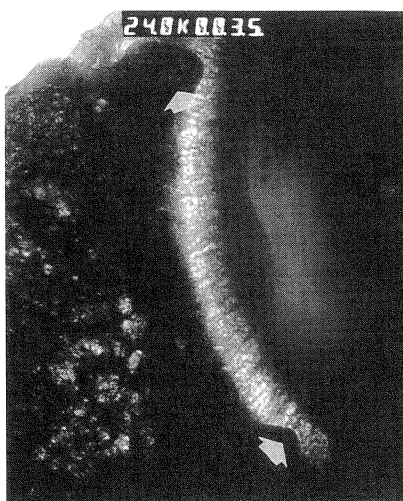
Fig. 5. Detail of a large PFA particle (right) with a rim of porous C-S-H, and another denser rim, containing mainly C-S-H, but also two areas consisting of Ca, Si, Al and Fe (possibly hydrogarnet; see arrows). Scale: 1 cm = 600 nm.
