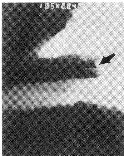
Fig. 8. Detail of the reaction zone surrounding a PFA particle, clearly displaying a dense C-S-H outer zone (arrow), and a porous C-S-H inner zone. Scale: 1 cm = 500 nm.
