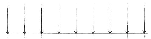
A slightly different case occurs when alternating bays carry a large and small load. Now the co-symmetric part is found by taking the average of the two loads, and the contra-symmetric part as the remainder after the average is subtracted. Again the words co-symmetric and contra-symmetric refer to the symmetry of the structure for translation over a distance equal to the length of one bay.
