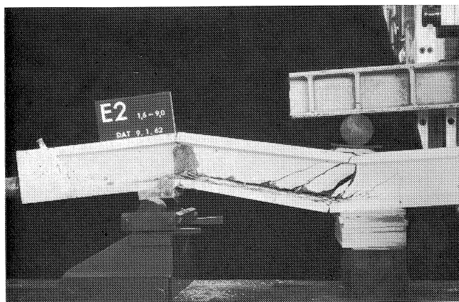
Fig. 60. Beam after failure in shear loading test.
